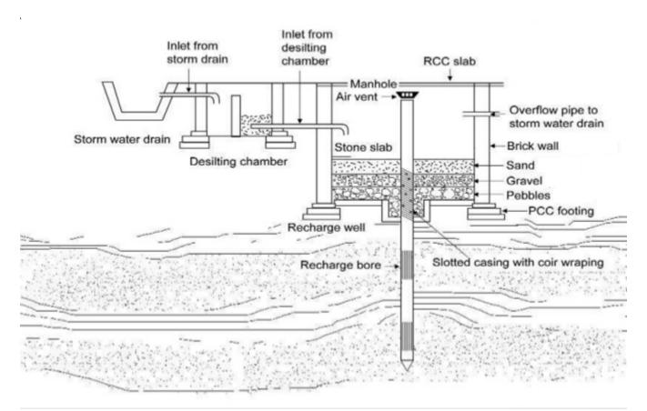
Recharge Pit Method is most suitable for such alluvial areas (plains) where permeable strata are not below than 2 to 2.5 meter deeper from the ground surface.
