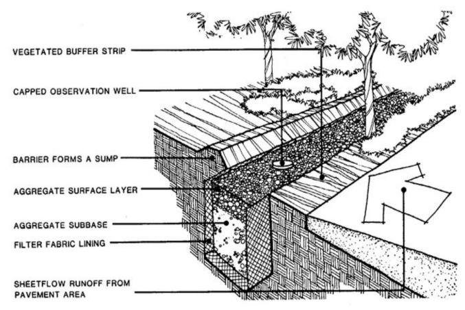
Recharge trench is also a simple method like recharge pit. Difference is only of shape and size.
