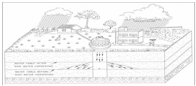
If the area of roof is 300 SQM and general rainfall is 700MM to 900MM, in this case rain water collected from rooves can be easily recharged through dry and open well.
